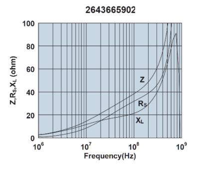
Impedance, reactance, and resistance vs. frequency.
