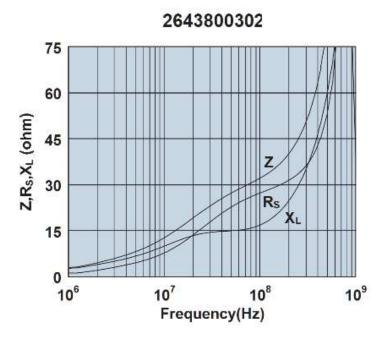
Impedance, reactance, and resistance vs. frequency.
