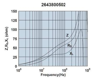
Impedance, reactance, and resistance vs. frequency.
