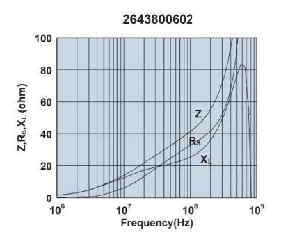
Impedance, reactance, and resistance vs. frequency.
