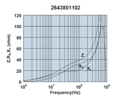
Impedance, reactance, and resistance vs. frequency.
