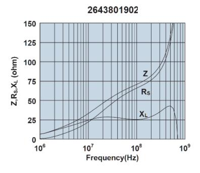
Impedance, reactance, and resistance vs. frequency.
