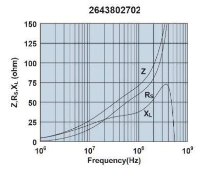
Impedance, reactance, and resistance vs. frequency.
