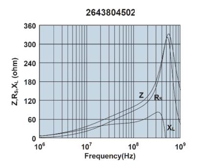
Impedance, reactance, and resistance vs. frequency.
