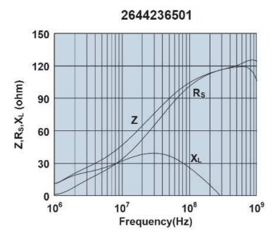
Impedance, reactance, and resistance vs. frequency.
