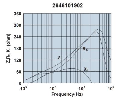
Impedance, reactance, and resistance vs. frequency.
