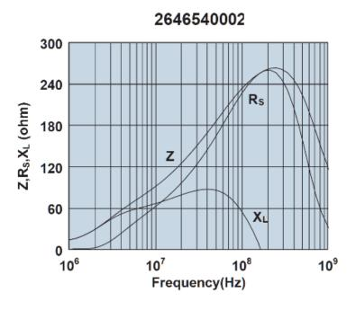
Impedance, reactance, and resistance vs. frequency.
