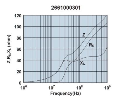
Impedance, reactance, and resistance vs. frequency.
