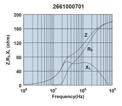
Impedance, reactance, and resistance vs. frequency.
