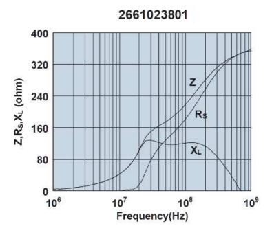
Impedance, reactance, and resistance vs. frequency.
