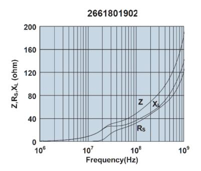
Impedance, reactance, and resistance vs. frequency.
