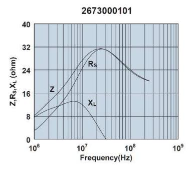
Impedance, reactance, and resistance vs. frequency.
