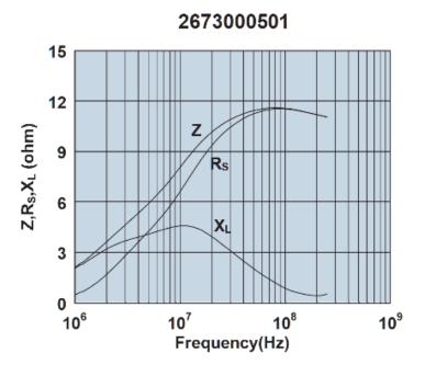
Impedance, reactance, and resistance vs. frequency.
