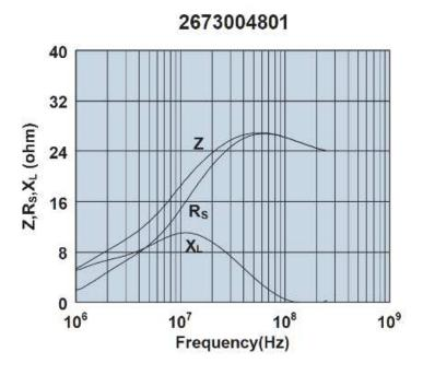
Impedance, reactance, and resistance vs. frequency.
