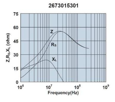
Impedance, reactance, and resistance vs. frequency.
