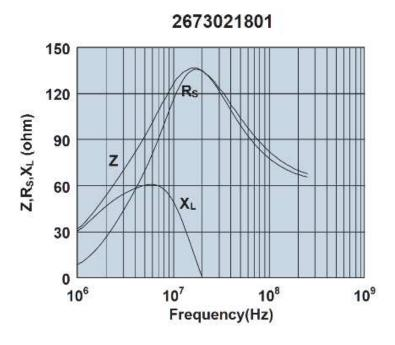
Impedance, reactance, and resistance vs. frequency.
