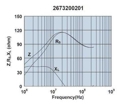
Impedance, reactance, and resistance vs. frequency.
