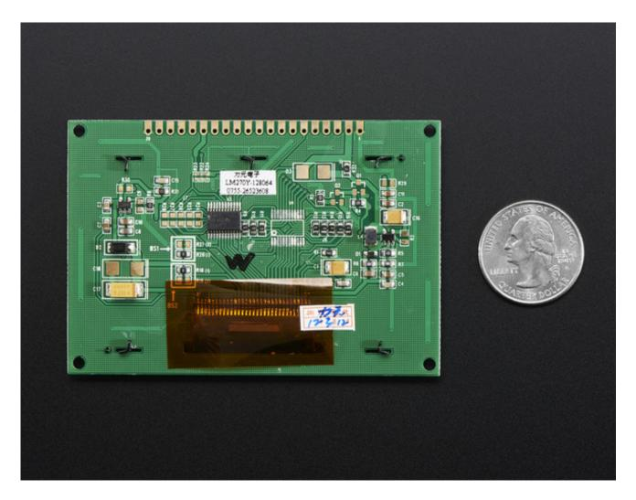
Getting started is easy! We have a detailed tutorial and example code in the form of an Arduino library for text and graphics. (http://adafru.it/iTb) You'll need a microcontroller with more than 1K of RAM since the display must be buffered. The library can print text, bitmaps, pixels, rectangles, circles and lines. It uses 1K of RAM since it needs to buffer the entire display but its very fast! The code is simple to adapt to any other microcontroller.
