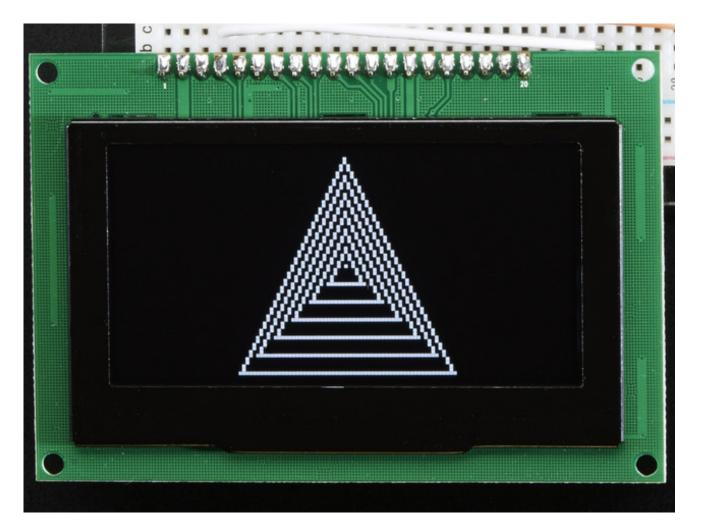
The power requirements depend a little on how much of the display is lit but on average the display uses about 50-150mA from the 3.3V supply. Built into the OLED driver is a simple switch-cap charge pump that turns 3.3V into a high voltage drive for the OLEDs.
