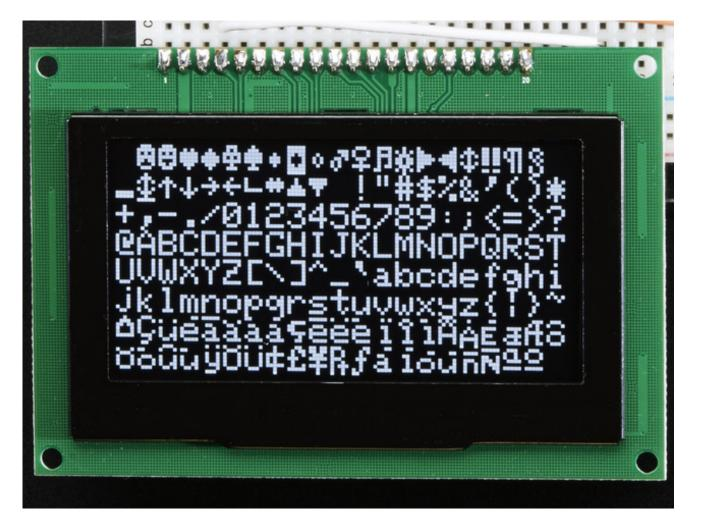
The driver chip, SSD1325 can communicate in two ways: 8-bit or SPI. Personally we think SPI is the way to go, only 4 or 5 wires are required. The OLED itself requires a 3.3V power supply and 3.3V logic levels for communication. We include a breadboard-friendly level shifter that can convert 3V or 5V down to 3V, so it can be used with 5V-logic devices like Arduino.
