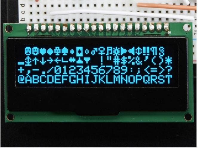
The driver chip, SSD1305 can communicate in three ways: 8-bit, I2C or SPI. Personally we think SPI is the way to go, only 4 or 5 wires are required and its very fast. The OLED itself requires a 3.3V power supply and 3.3V logic levels for communication. We include a breadboard-friendly level shifter that can convert 3V or 5V down to 3V, so it can be used with 5V-logic devices like Arduino.
