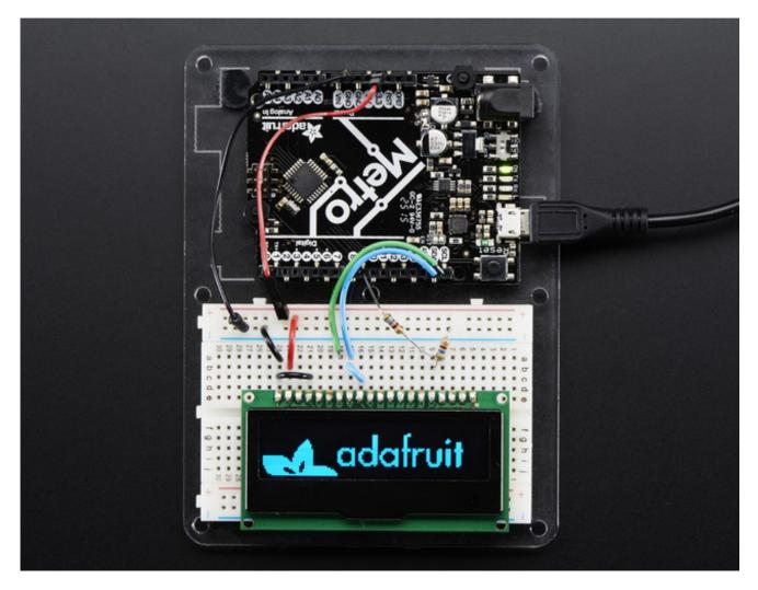
Don't forget you have to set the display to I2C mode, see the Assembly step on how to do that!
