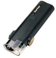
Item # 26800C-538, Illuminated Pocket Microscope 30x with Scale: Measuring Range 4 mm, Graduation 0.1 mm
