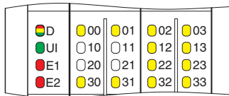
Figure 8 Local diagnostic and status indicators
