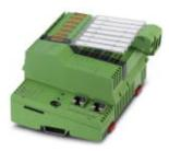
Inline controller with integrated pulse/direction/PWM interface, RS-485/RS-422, analog inputs (0  $\dots$  10 V), and analog outputs (0  $\dots$  10 V), with programming options according to IEC 61131-3
