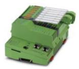
Inline controller with integrated pulse/direction/PWM interface, RS-485/RS-422, fast counters, and incremental encoder inputs, with programming options according to IEC 61131-3
