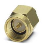
The termination resistor is screwed onto an unused antenna connection of a WLAN device, e.g., in leaky wave applications. This terminates the connection with the correct impedance and prevents undesirable emission.
