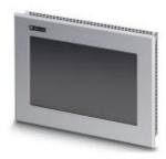
Touch panel with 17.8 cm (7.0") graphics-capable TFT display, 65,535 colors, 800 x 480 pixels, 1 x Ethernet, 1 x MPI, 2 x USB, and integrated runtime of the Visu+ visualization software
