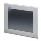
Touch panel with 30.7 cm (12.1") graphics-capable TFT display, 65,535 colors, 800 x 600 pixels, 1 x Ethernet, 2 x USB, and integrated runtime of the Visu+ visualization software.
