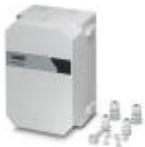
Control box for rugged construction of wireless systems for industrial applications, IP65, 25 x 18 x 13 cm, polycarbonate material, gray, drilled, including DIN rail, plugs, and screw connections, without devices
