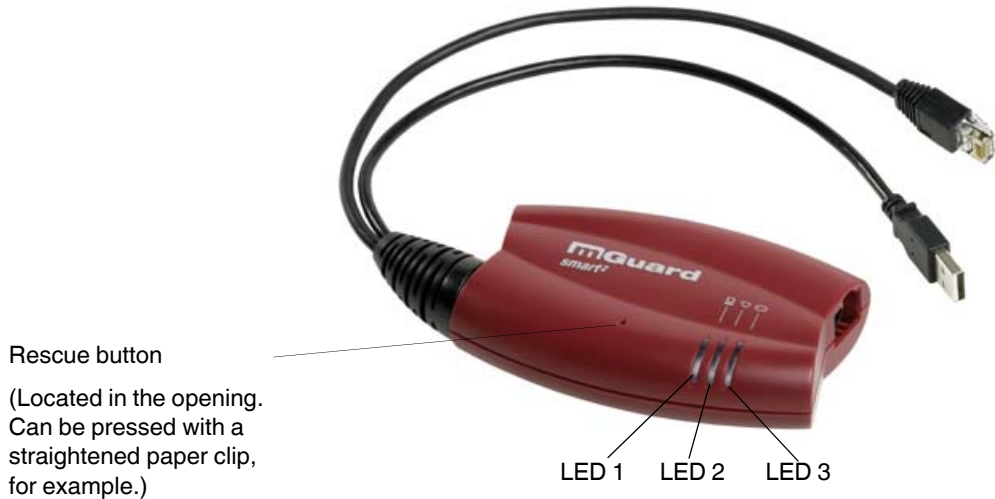
Figure 2-2 Operating elements and LEDs on the FL MGuard SMART2
