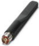
Omnidirectional antenna, 2.4 GHz/5 GHz, gain: 2.5 dBi/5 dBi, polarization: linear, opening angle: h/v 360°/30°/16°, degree of protection: IP68, connection: N (male), corresponding connecting cable for control cabinet feed-through (Order No. 2701402)
