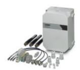
Control box set for constructing wireless systems for industrial applications, incl. three 2.4/5 GHz omnidirectional antennas that can be directly screwed on, IP66, with DIN rail, plugs, and screw connections, with 100 ... 240 V power supply unit, without devices
