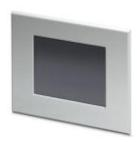
Touch panel with 14.5 cm/5.7" TFT active-display (Resistive industrial touch screen), 320 x 240 Pixel(s) (QVGA), 65536 colors, ARM9<sup>™</sup>, 184 MHz, 2x USB host 2.0, 1 x Ethernet (10/100 Mbps), RJ45, Windows CE 5.0 and user software: MicroBrowser. (bus system: without)
