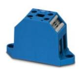
Device terminal block, Connection method: Screw connection, Number of positions: 1, Cross section: 0.5 mm² - 16 mm², AWG: 20 - 6, Width: 24.8 mm, Height: 40 mm, Color: blue, Mounting type: Screw mounting
