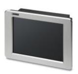
Touch panel with 38.1 cm/15" TFT-Display (Resistive industrial touch screen), 1024 x 768 Pixel (XGA), 65536 colors, Intel<sup>®</sup> Celeron<sup>®</sup> M ULV 423 1.01 GHz, COM 1 (RS-232), 1x VGA, 4x USB, 2x CompactFlash<sup>®</sup>, 2x Ethernet (10/100/1000 Mbps), RJ45, Windows CE 6.0 and User software: Visu+ / AX OPC Server. (Bus system: without)
