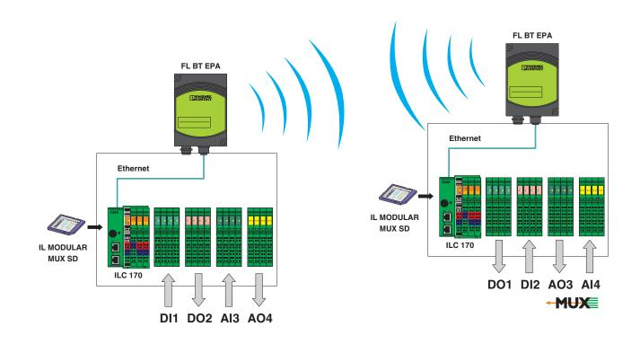
The software on the SD FLASH 512MB MODULAR MUX CompactFlash<sup>®</sup> card transforms the ILC 131 ETH and the individual input and output terminals required into a flexible field multiplexer. As a wireless connection or as a point-to-point connection in an Ethernet network.
