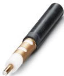
The leaky wave cable is a "wireless cable" which acts as an antenna and emits along its entire length. The range is limited. Track-guided systems, for example, can therefore be supplied as required, even under difficult conditions. Suitable for the 5 GHz band.
