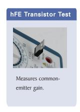
The 2704C has all of the functionality for basic DMM applications including some high end features you might not expect. The 2000 count LCD can display resistance values up to 2 G $\Omega$ , capacitance to 20 uF or a transistors common-emitter gain value up to 1000. Value-packed features make this meter a must in every "Tool Kit\*".
