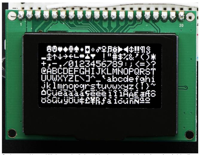
Getting started is easy! We have a detailed tutorial and example code in the form of an Arduino library for text and graphics. You'll need a microcontroller with more than 512 bytes of RAM since the display must be buffered. The library can print text, bitmaps, pixels, rectangles, circles and lines. It uses 512 bytes of RAM since it needs to buffer the entire display but its very fast! The code is simple to adapt to any other microcontroller.
