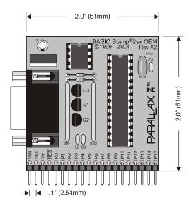
The BASIC Stamp 2sx is available in the above two physical packages. The BS2sx-IC (Figure 1.7) uses surface mount components to fit in a small 24-pin DIP package. The preassembled BASIC Stamp 2sx OEM (Figure 1.8) features an easier-to-trace layout meant to aid customers who wish to integrate the BASIC Stamp 2sx circuit directly into their design (as a lower-cost solution). The BASIC Stamp 2sx OEM is available in assembled form only.
