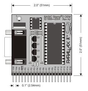
The BASIC Stamp 2 is available in several physical packages. The BS2-IC (Figure 1.4) uses surface mount components to fit in a small 24-pin DIP package. The BASIC Stamp 2 OEM (Figure 1.5) features an easier-to-trace layout meant to aid customers who wish to integrate the BASIC Stamp 2 circuit directly into their design (as a lower-cost solution). The BASIC
