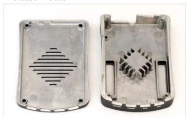
The ALU case is designed in a way that serves entirely as a big heat sink. On the interior part of the housing there is a large 16x16x12mm block which is directly connected to the FPGA of the STEMlab and in this way passes all the heat to the housing.
