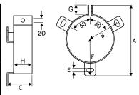
When using mounting clamps, care should be taken not to obscure any safety vent in the can. Delivered without bolts and nuts for mounting. PYC clips are for PEH169 and PEH200 capacitors.
