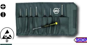
273 99 Set 8 Pcs. Slotted & Phillips Precision ESD Safe Dissipative Handle. Blade high alloy CVM steel, hardened, hard chromed. Handle manufactured from impact resistant, dissipative material. In storage pouch ESD standard IEC 61340-5-1
