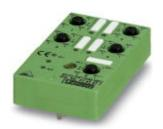
Passive signal distributor, connection element, from flat-ribbon cable to 5 x M12 plug, e.g., for connecting up to 5 FLX AS-i M8 devices or 5 AS-i S-Line devices to the AS-i flat-ribbon cable
