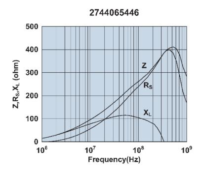
Impedance, reactance, and resistance vs. frequency.
