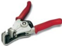
Stripping pliers for transmitting individual elements of the fiber optic cable. Especially suited for all polymer and HCS cables. Special mechanics and precise blade form avoid damage to the fiber optic fibers. Dimensions: (L x W x H) 160 x 130 x 36 mm.
