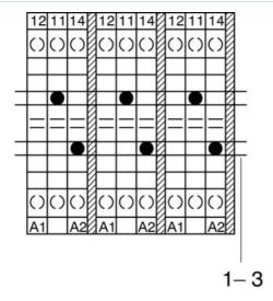
1-3 = fixed bridge, cross connection rail, spacer
