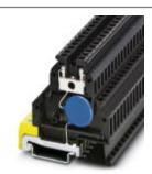
Modular terminal block with varistor as surge voltage protection between clamping connector and DIN rail, separate ground connection, nominal voltage: 48 V DC, mounting on NS 35/7.5, terminal width: 6.2 mm, terminal height: 69 mm
